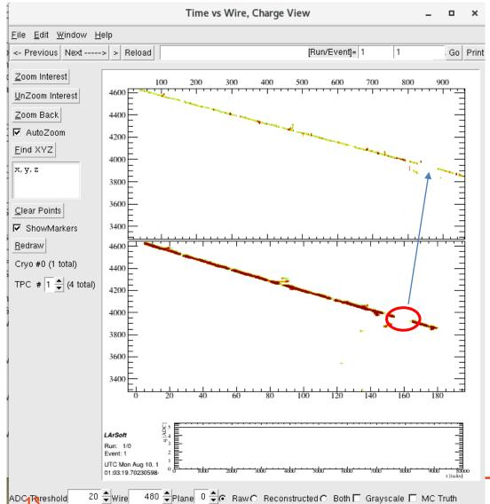
Masked channels in this view due to LEM border No charge is also collected in the other view for this region as it should be
