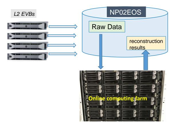
→ Short time interval in between the assembly of a file by one event builder and the availability of the reconstruction results is ~15 minutes
