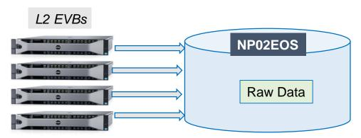
The raw data files assembly by the event builders and their transfer to NP02EOS is done with a **dedicated software**, which has developed taking into account the network configuration and the characteristics of the EVBs. This software has been intensively tested since 2018 with dedicated data challenges and it has been ensuring smooth data handling in 2019
