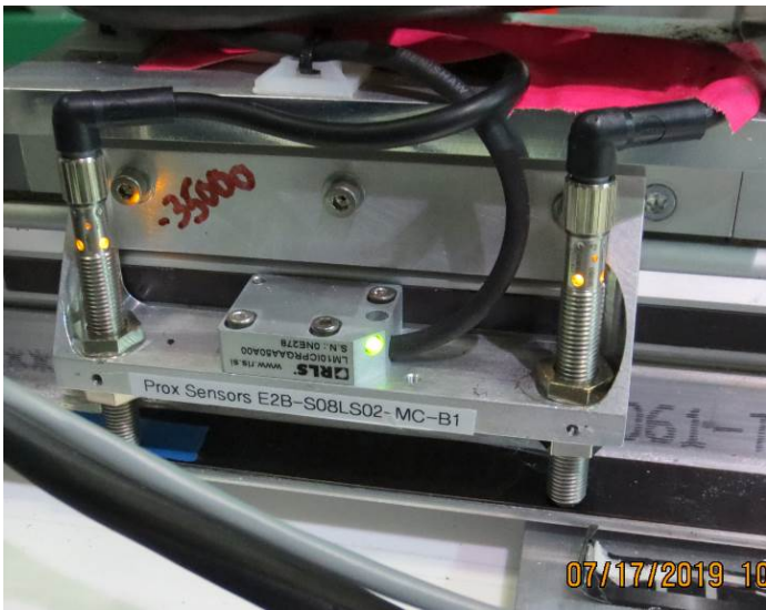
Figure 3: Encoder to provide Z-axis position reading, 2 proximity sensors to ensure height is okay.
