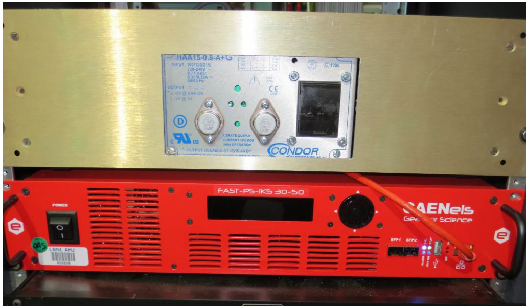
Figure 2: Power supply for the magnet and current monitor for the power supply to the magnet
