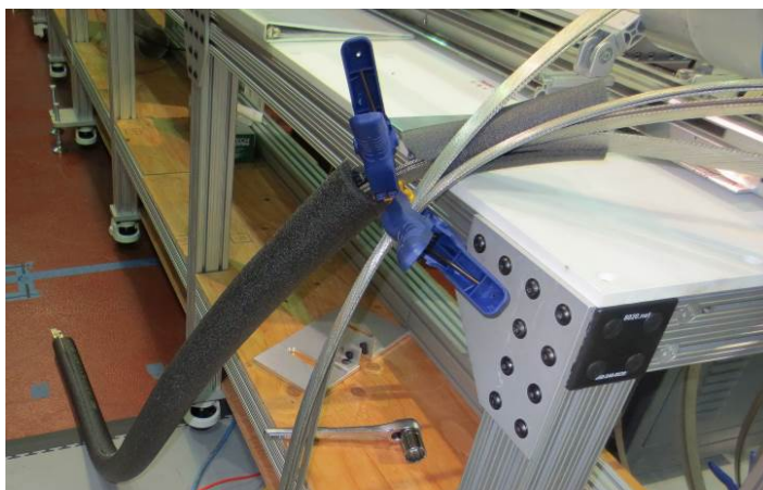
Figure 4: One set of leads wrapped in pipe insulation
