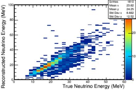
Correcting the total observed amount of photons for the average number of photons expected per MeV as a function of position along the drift direction.
