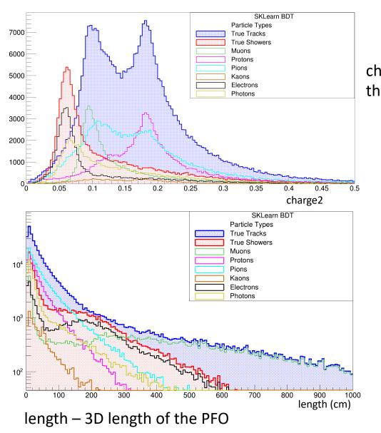
the UNIVERSITY OF WARWICK charge2 – Ratio of charge in the last 10% of the PFO and the mean charge in the collection plane
