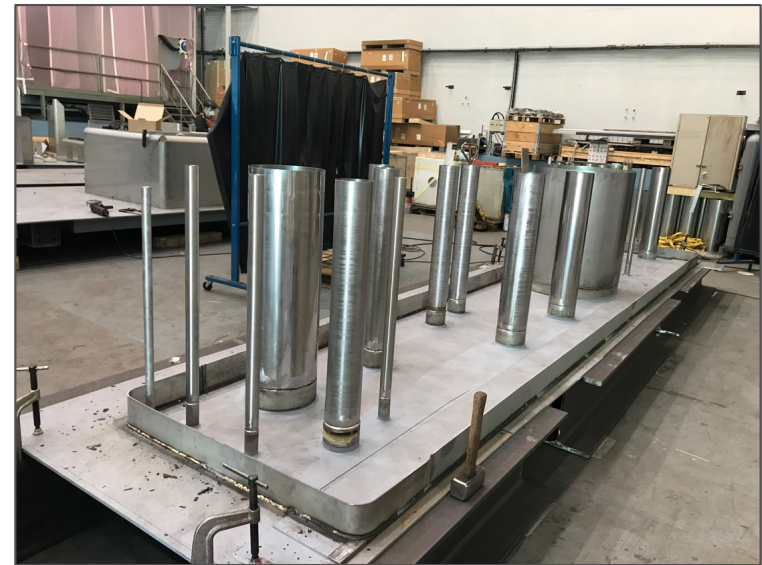
Cryogenics top cap fabrication
