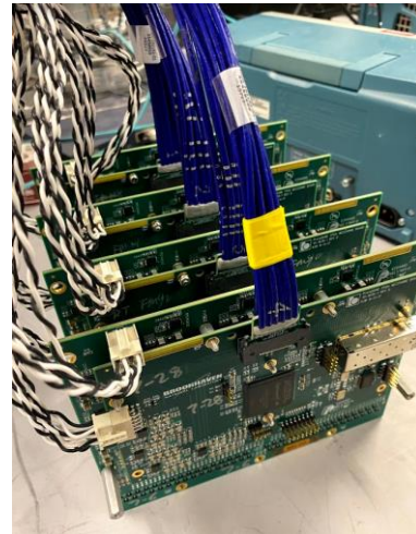
WIB standalone read-out supports up to 4 FEMBs
