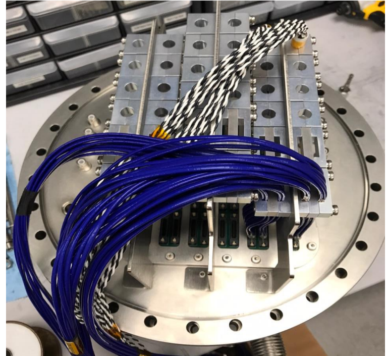
Cables + strain relief on cold flange side
