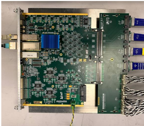
WIB standalone read-out supports up to 4 FEMBs
