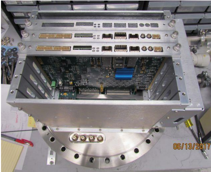
Crate with 2 WIBs on warm flange side
