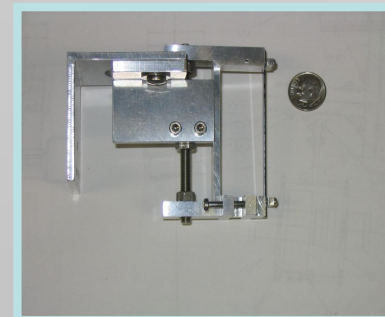
Strip type crystal 1mm wide X 3mm long 150 urad bend angle (INFN, IHEP)
