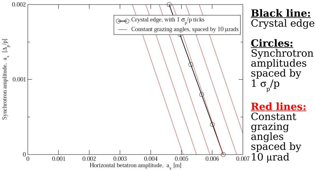
UA9 looks ok: the grazing angle changes by only 0.48  $\mu$ rad per  $\sigma_p/p$ , despite large negative dispersion at the crystal.
