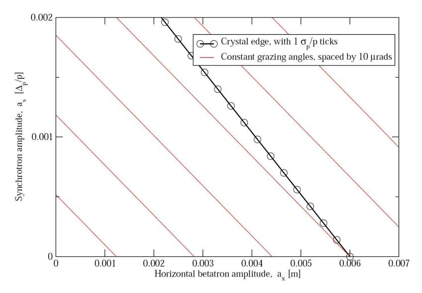
Flattened slopes: grazing angle changes by 0.41 µrad per 3  $\sigma_{_p}/p.$  Measured optics values also available.
