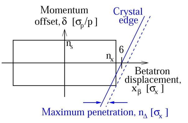
A "grazing particle" just touches the crystal during simultaneous betatron & synchrotron oscillation extrema.
