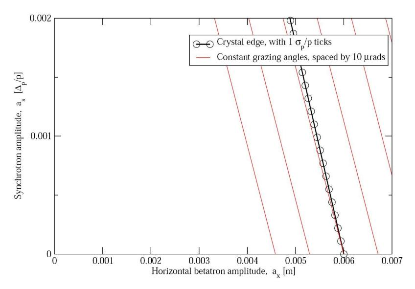
Small  $\sigma_p$ /p, small channeling acceptance: grazing angle changes by only 0.11 (0.31)  $\mu$ rad per  $\sigma_p$ /p at 7 (0.45) TeV.
