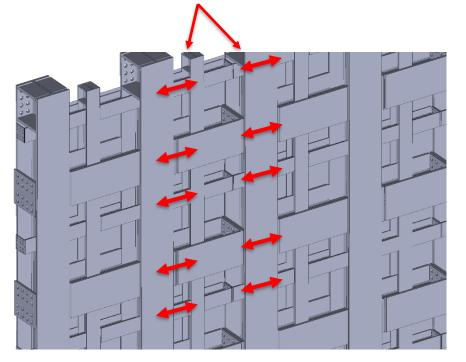
Weld seams on backside to form • moisture barrier
