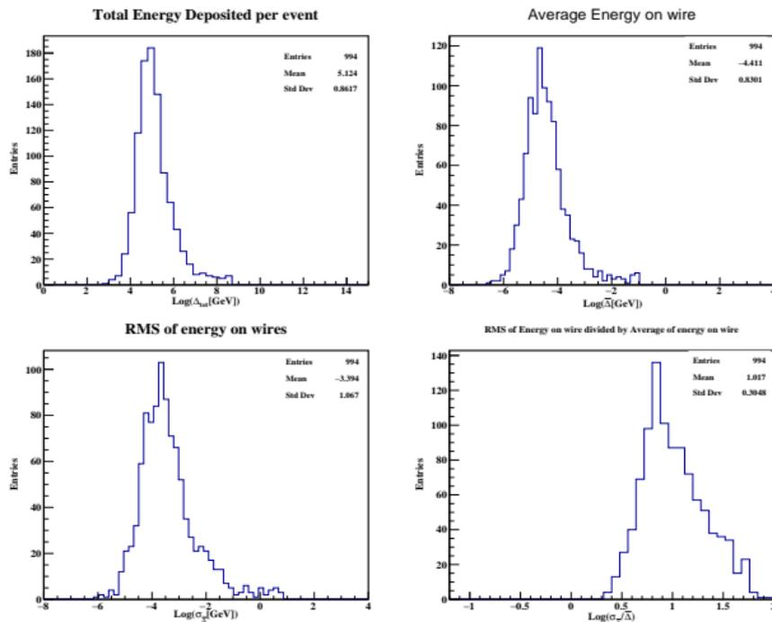
Figure 2 : Histograms for 10 TeV muons events in LArTPC, similar histograms for other energies can be found at : [▶ Histograms](#)
