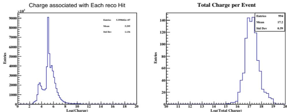
Figure 7 : Left panel shows the Log of Charge at collecting wires planes associated with each reconstructed hit. Right panel show the log of total charge per event for 10 TeV muons events in LArTPC.
