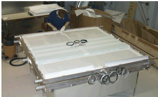
Large-area plastic scintillator internals
