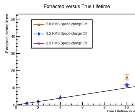
Figure 2: "Space charge Off" results for 1-10ms lifetimes.
