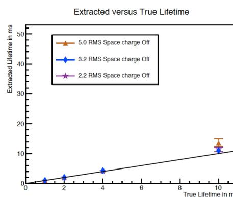
Figure 4: "Space charge Off" results for 1-10ms lifetimes with the lowered hit threshold.
