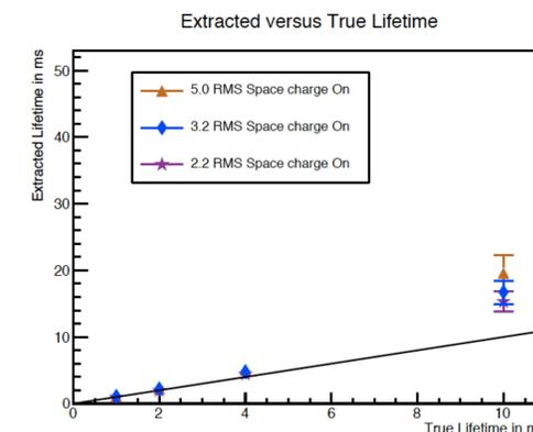
Figure 5: "Space charge On" results for 1-10ms lifetimes with the lower hit threshold.
