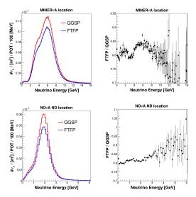
→ Energy peak is around 6 GeV for MINER $\nu$ A, and 2 GeV for NO $\nu$ A ND locations which agrees with the equation on slide 6. → QGSP predicts higher  $\nu_{\mu}$  flux than FTFP by ~ 15%.
