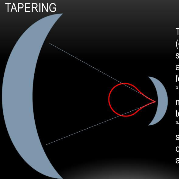
To minimize side lobes (caused by diffraction at sharp edges) the antenna pattern of the feed is often designed to "underilluminate" the main dish. This technique, called "tapering" minimizes sidelobes at the expense of a slight degradation in angular resolution.
