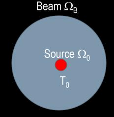
The antenna temperature is the average brightness temperature of the source, "diluted" by the ratio of the source solid angle to the beam solid angle.
