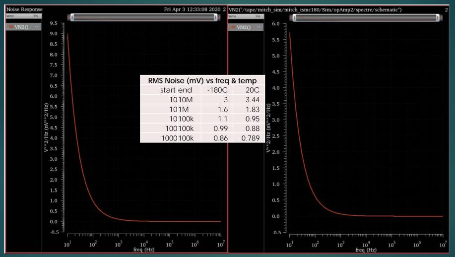
April 3, Results with finer settings of SPICE convergence options \*\*1P $\Omega$  noisless resistor holds across integrator
