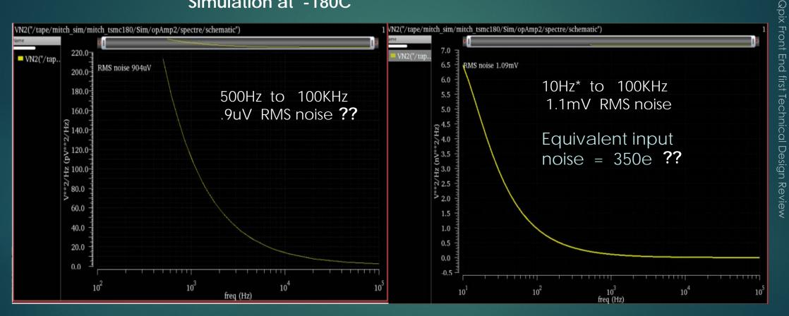
\* Note 10Hz has significant attenuation with this test bench
