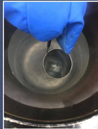
Photo 6: Dipping the PCBs into liquid Ar
