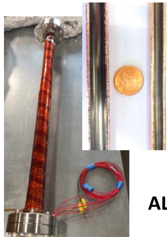
Insertion device chamber (d=6mm)
