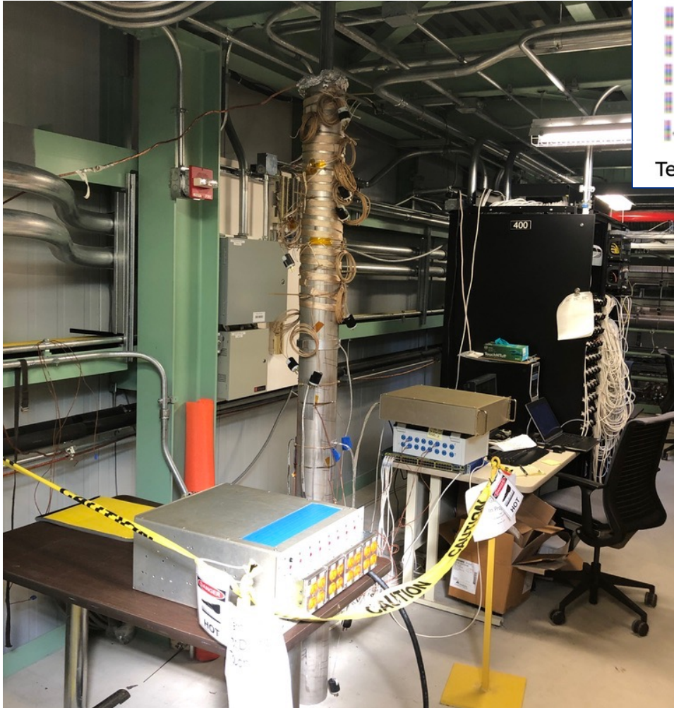
16-channel bake test setup.
