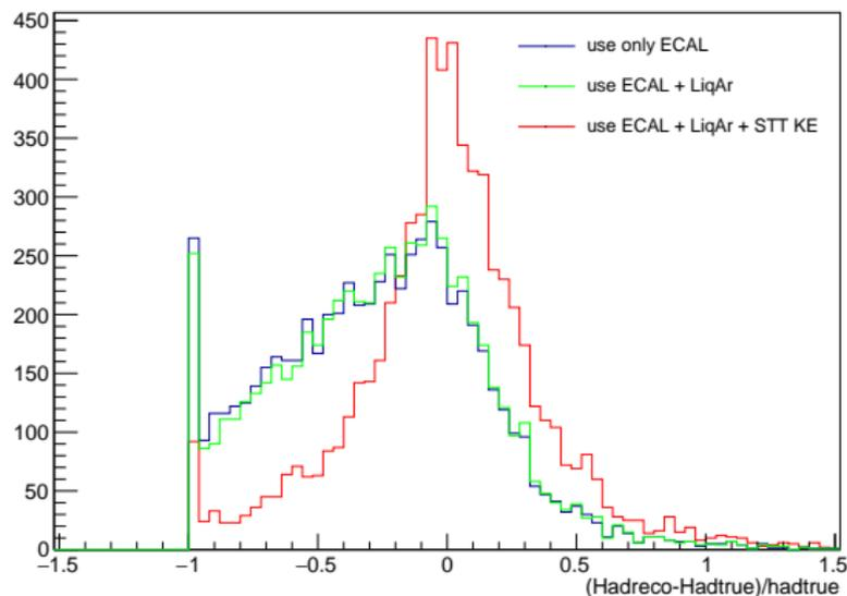
Substantial leakage from ECAL recovered by STT
