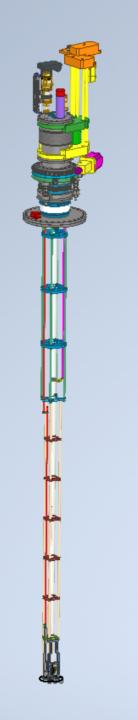
Alternative idea for electrical insulation for the laser periscope
