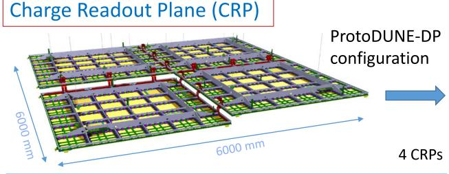
2 instrumented CRPs with 36 LEMs and 36 anodes (50x50 cm<sup>2</sup>):
