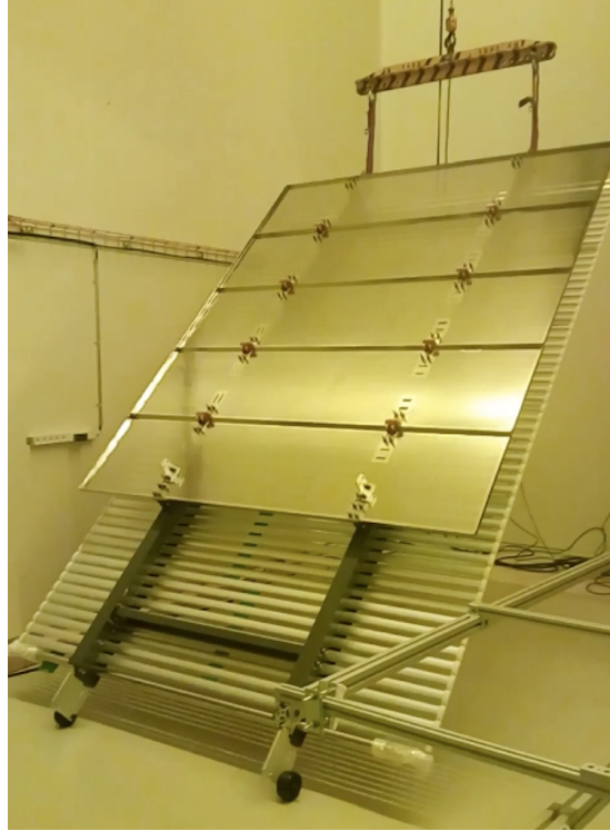
Figure 6. Lifting of a Top FC module. The latches that connect to the APA are at the bottom.
