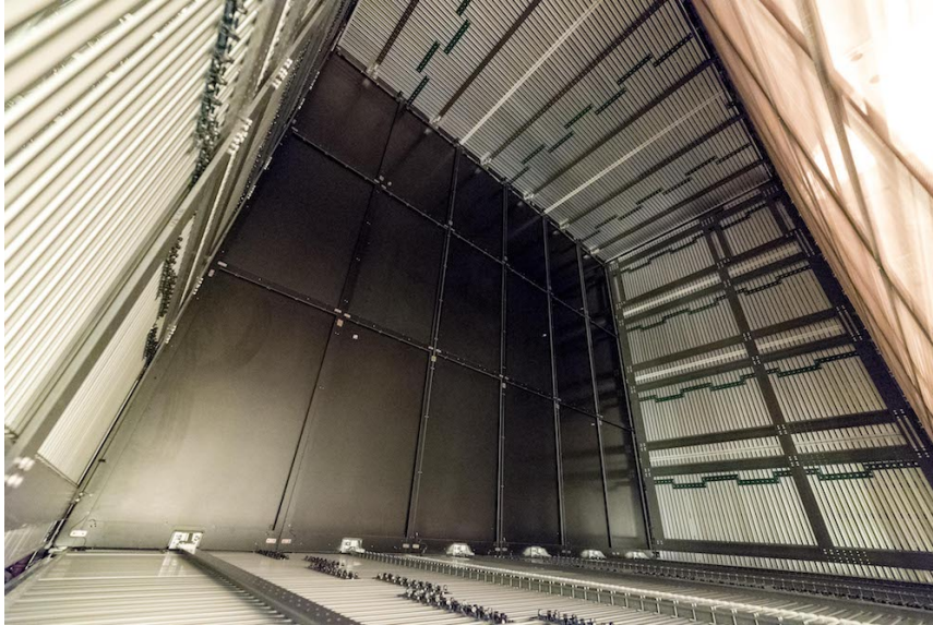
Figure 2. One of the two drift volumes of ProtoDUNE-SP. The FC modules enclose the drift volume between the CPA array (at the center of the image) and the APA (upper right). The endwall FCs are oriented vertically; the top and bottom units are horizontal. The staggered printed circuit boards connecting the endwall FC profiles are the voltage divider boards.
