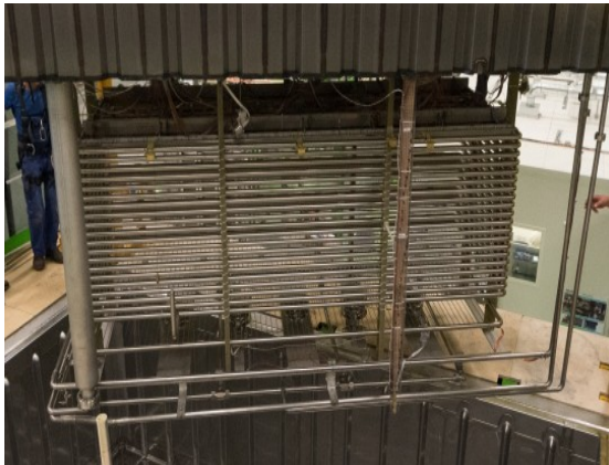
WA105 3x1x1 m3 (CERN): 2014-2017. 5 ton LAr. 1m drift. JINST 13 (2018) P11003
