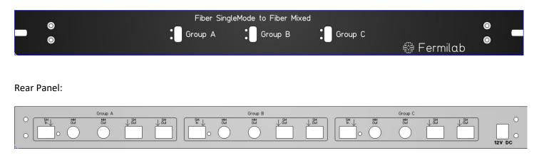
The Fiber SingleMode to Fiber Mixed has 3 groups of receivers. Each group takes in a 1300nm SingleMode Fiber signal that is then distributed to 2 MultiMode Fiber channels and 2 SingleMode Fiber channels on the rear panel. The Fiber input is also transmitted back out the SingleMode Fiber output of the transceiver, so daisy chaining systems via fiber is possible. The front panel contains 2 lemo style 50 Ohm TTL monitor outputs of each of the channels as well.
