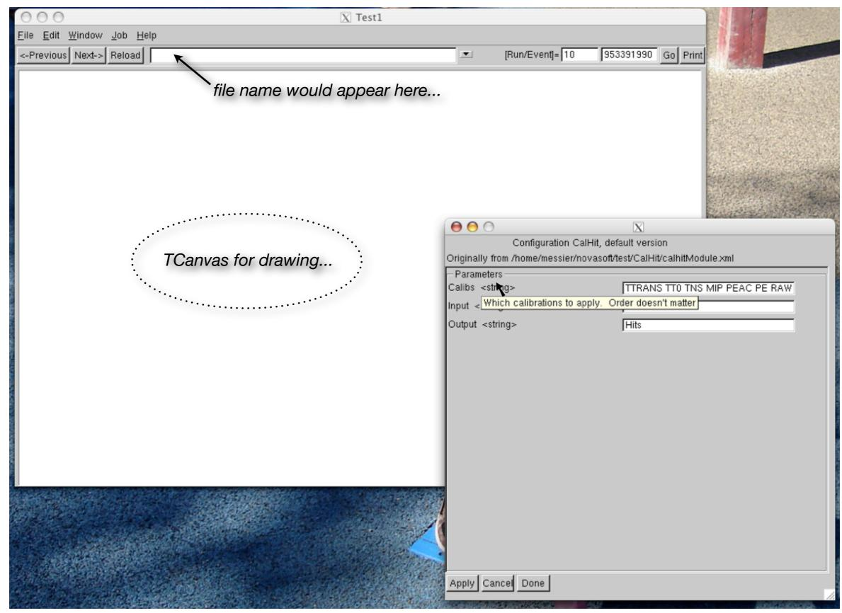
Screen shot of the window provided by the EventDisplayBase package (program: test\_evdb). The dialog window was launched by selecting "Job/Edit Config" and shows how to edit module configurations. Hitting "Apply" would cause any reconstruction to be re-applied and the event re-displayed. User's are responsible for filling the big blank window with some representation of the data from their detector.
