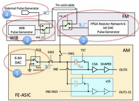
Measurements with LArASIC/FPGA DACs repeated during ProtoDUNE data taking
