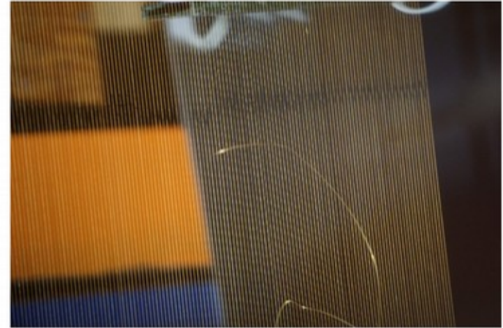
Figure 8. Photograph of a broken wire on the test setup. The wire was cut at its bottom attachment point and can easily be spotted because it is curling up and distorting the wire pattern. Note that only one plane of vertical wires is strung in this particular test.
