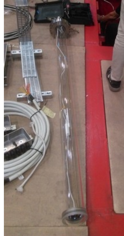
PDSP inspection camera in acrylic tube before installation
