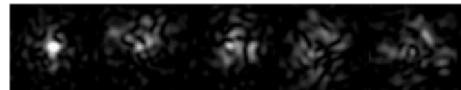
“Speckle” due to temperature fluctuations in turbulent gas flow. (In air, not LAr.)
