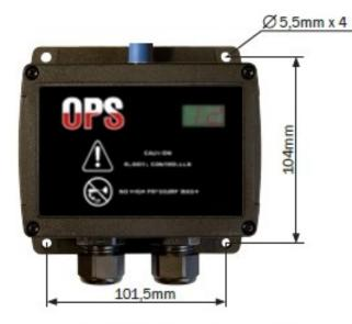
The Central Unit should be installed vertically or horizontally with cable glands facing downwards or horizontally. The Central Unit should never be assembled with cable glands facing upwards or in any ways where it is exposed to accumulation of water, moisture, and other debris.
