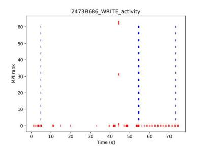
Provides details on each I/O operation issued by each rank, providing a complete picture of which ranks are performing I/O and how long they are spending on I/O
