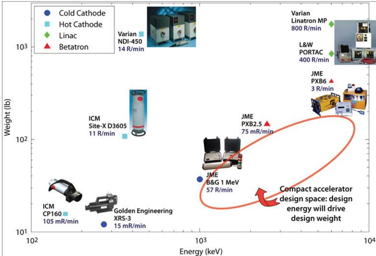
PORTAC is commercial state-of-the-art 6-MeV accelerator (300 R/m/min)
