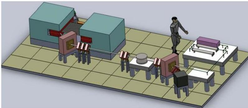
The 150-MeV Sumitomo Heavy Industries RTM has size 4m by 1.5m by 2m, excluding the injector line from the electron gun, using 1.2 T magnets. Their design concept for a 220-MeV RTM for generation of high-energy gamma rays for SNM detection using inverse Compton scattering for a JAEA project uses 1.5 T dipoles.
