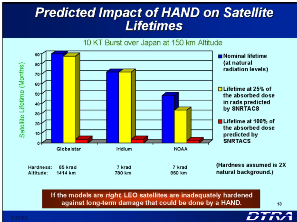
Typical low LEO satellites (~800 km) are designed to tolerate ~ 5 krads and high LEO satellites (~ 1400 km) are designed to tolerate ~ 50 krads. For 10 kT detonation at 150 km, enhanced flux leads to about 2.3 krad/month at 800 km.
