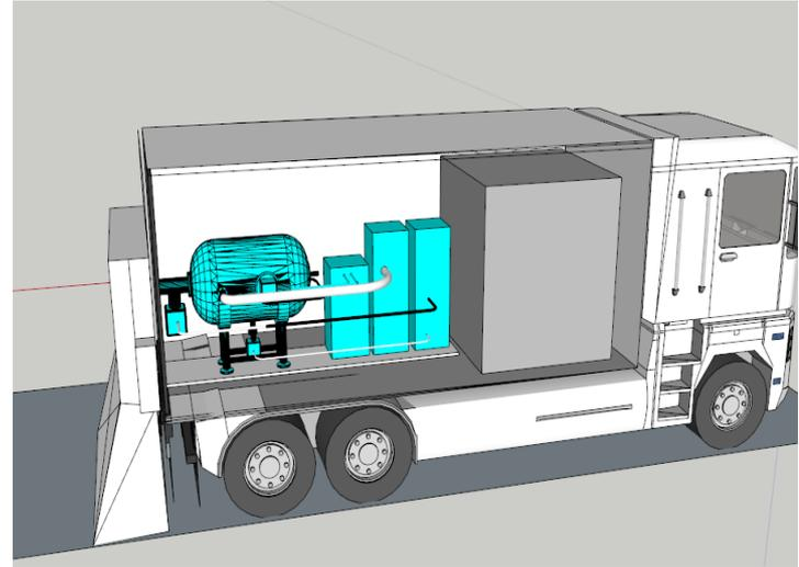
**Conduction cooling with 4K cryo-coolers (5W) and highly efficient RF drive**
