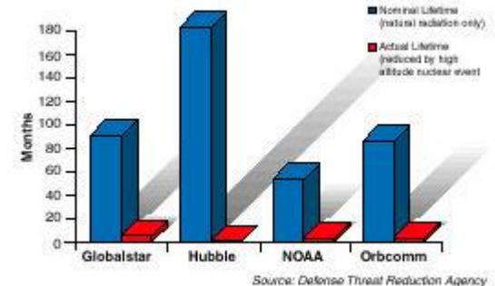
Figure 13: Impact of a nuclear detonation on the lifetime of satellites
