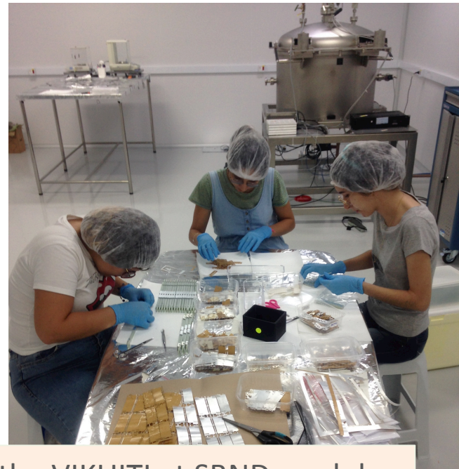
Gluing the VIKUITI at SBND modules
