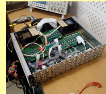
matching amplifier between ADC & preamplifier (IHEP)
