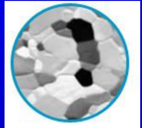
Example of FIB secondary electron imaging of grain boundaries of a specimen
