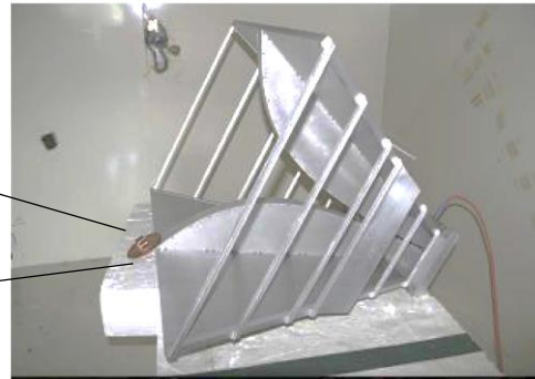
Fig. 3. Comparison of the 570-MHz small ground plane Z antenna and the dual-ridged reference horn in the NIST-Boulder reverberation chamber.
