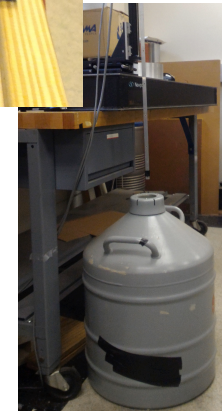
LN2 Dewar with temp control/ monitoring
