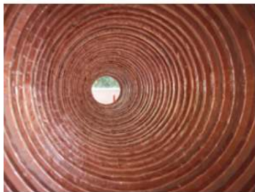
2 m horn with 78 sheets of 25 mm thick foam
