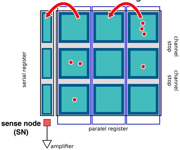
Shift charge in serial register one pixel down (3 times)
