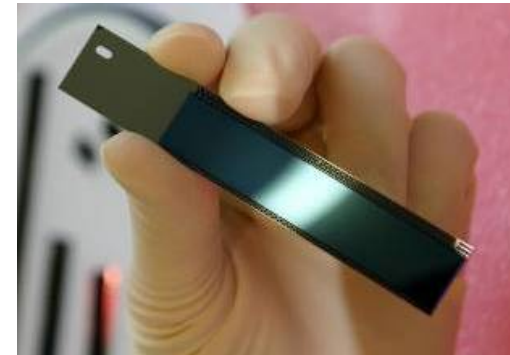
Thin (50µm-75µm) self-supporting all silicon module
