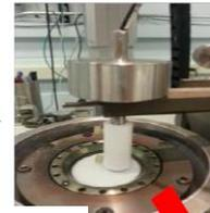
Pin-on-disc high vacuum tribometer
