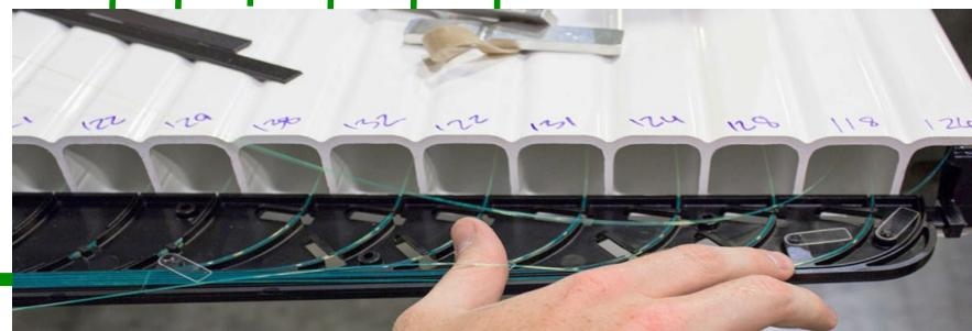
Each cell has loop of wavelength shifting fiber read out in groups of 32 by a 32 pixel Avalanche Photodiode
