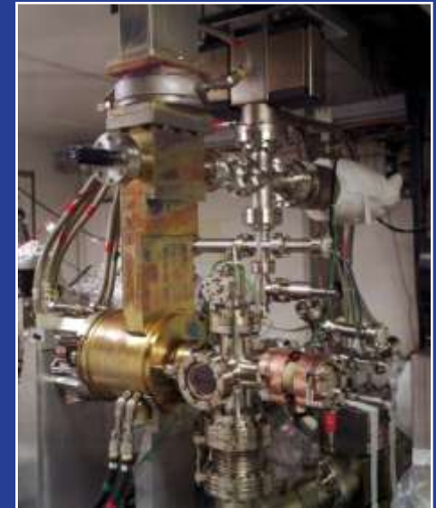
Existing FNAL RF gun; FNAL replace this cavity to modified DESY design.
