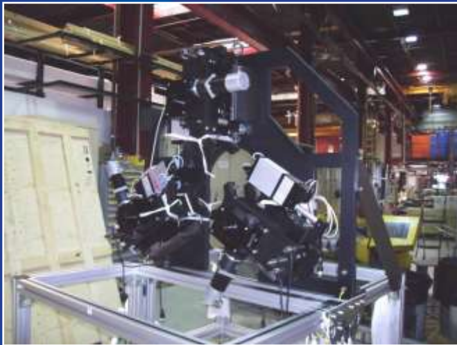
4 motorized cavity tuning devices fabricated during JFY07 (photo shows the one at Fermilab delivered on February 2008)
