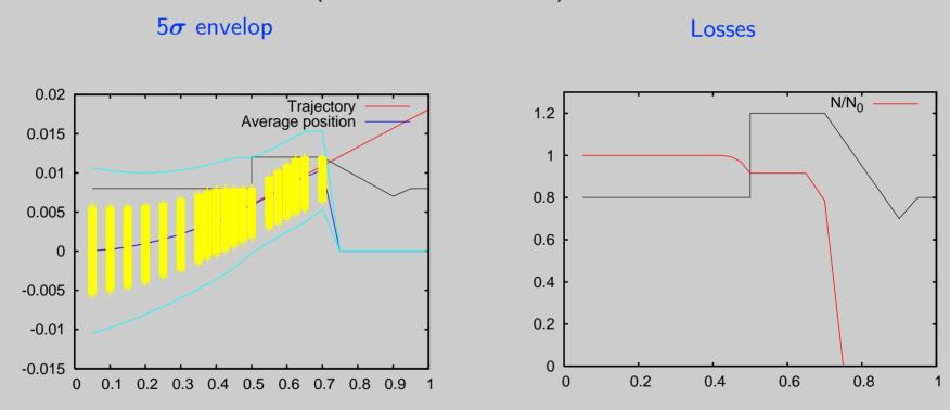
About 10% of the particles is lost on the upper chopper plate.
