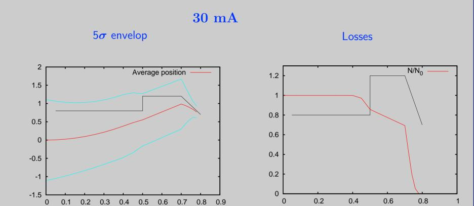
About 15% of the particles is lost on the upper chopper plate.
