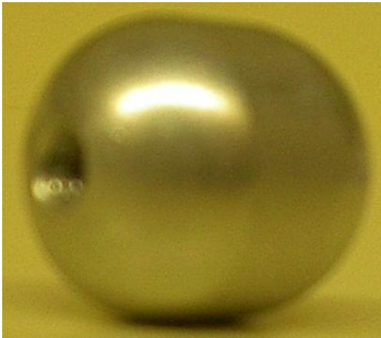
Figure 10: aluminum sphere with dia. of 0.8 inches used to tune the frequency of the
