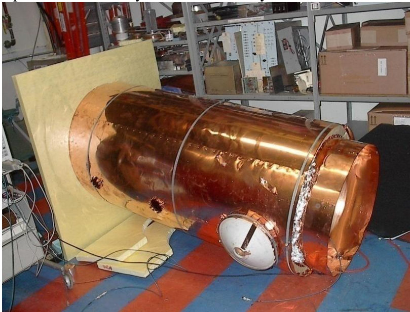
Figure 5: Prototype cavity after assembly with a polystyrene board for support.
