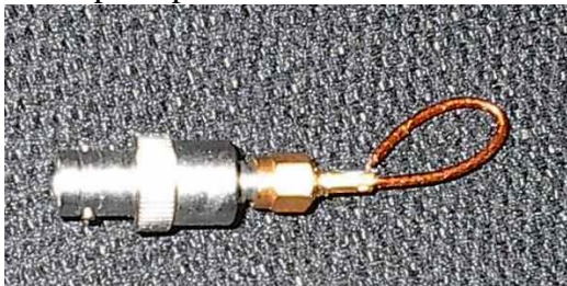
Figure 14: Power coupler pickup loops, used to measure the modes in the cavity.
