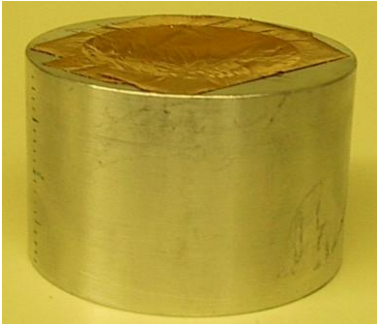
Figure 8: aluminum cavity tuner with dia. of 3.2 inches used to tune the frequency of the cavity.
