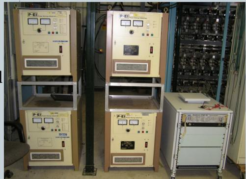
20Kw PEI Power Supplies 200V@100A each with a filter.
