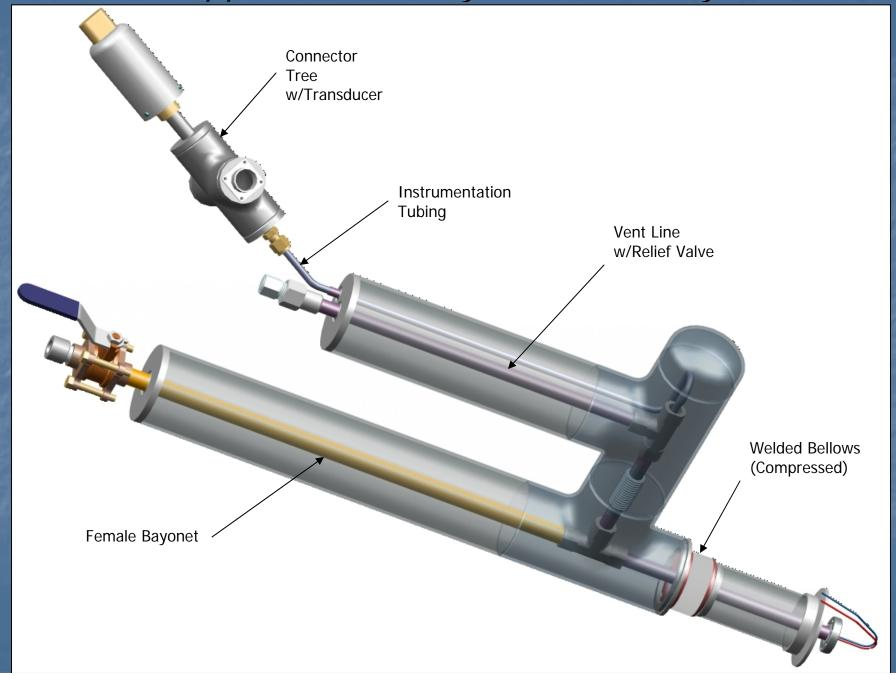
**Insert Current Lead-HTS** Conductor Assembly (Includes 4-Lower Bayonet Assemblies) on Strongback Channel 0
