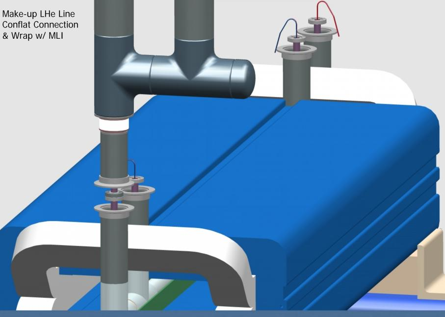
Make-up Vacuum Jacket Connection & Repeat for Remaining 3-Ports
