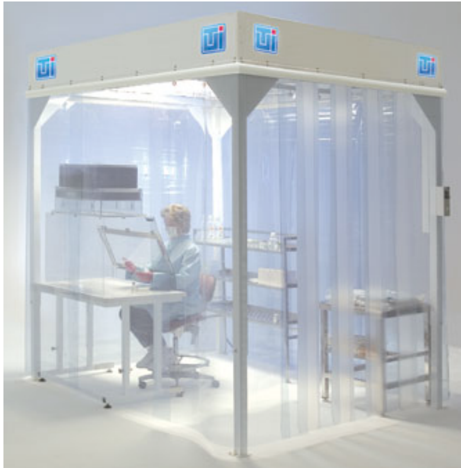
Figure 18: One large version of the portable clean room and two small versions will be used while accessing the clean optics inside the vacuum service vessels. Laminar flow from the ceiling maintains a clean environment, once loose debris and dust is cleaned from the floor. Monitors inside each of the clean rooms will ensure that the system is working as expected after a move, before we open the vessel to access clean optics.
