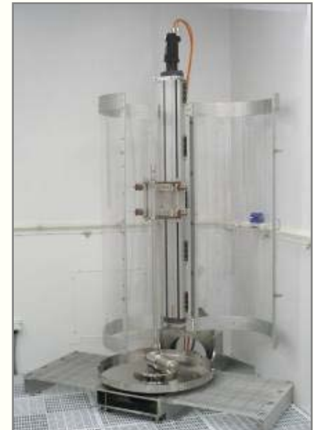
New High-pressure rinse system
