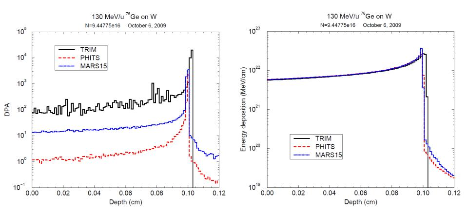
Pencil beam, uniform in R=0.03568 cm disc. Target  $W_{nat}$ , cylinder with R=0.03568 cm, L=0.12 cm
