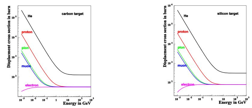
All products of elastic and inelastic nuclear interactions as well as Coulomb elastic scattering (NIEL) of transported charged particles (hadrons, electrons, muons and heavy ions) from 1 keV to 10 TeV contribute to DPA in MARS15 model.
