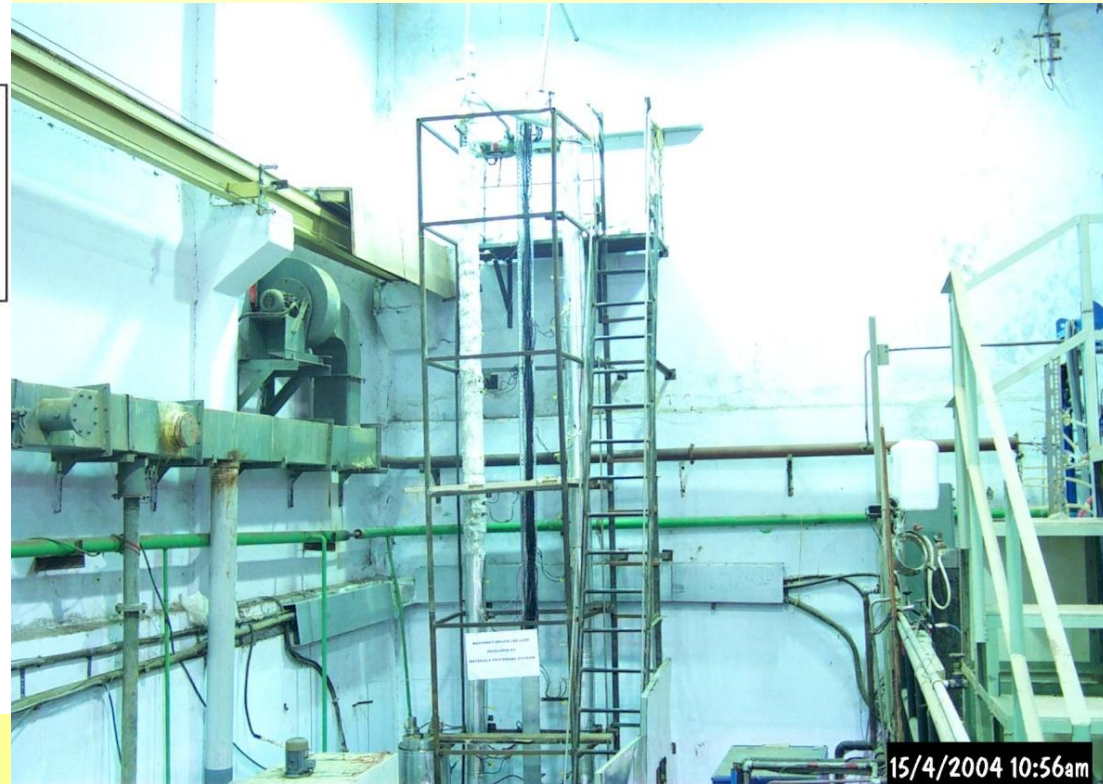
Gamma ray void fraction measurement system
